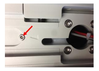
Figure 7. Stopper on a dovetail saddle
